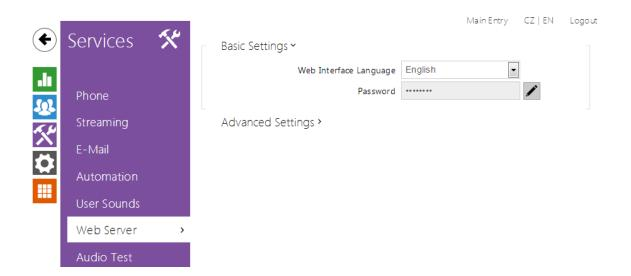
You can configure your  $2N^{\otimes}$  Helios IP intercom using a standard browser which accesses the integrated web server. Use the secured HTTPS protocol for communication between the browser and intercom. Having accessed the intercom, enter the login name and password. The default login name and password are **admin** a nd 2n respectively. We recommend you to change the default password as soon as possible.
