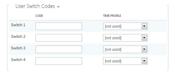
Each user can be assigned a private switch activation code. The user switch codes can be arbitrarily combined with the universal switch codes defined in the **Hardware** | **Switches** menu. If the codes are identical with the codes already defined in the intercom configuration, the mark will appear at the colliding codes.
