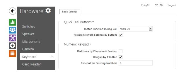
This configuration section helps you set the numeric keypad and quick dial button functions.  $2N^{\otimes}$  Helios IP allows you to:
