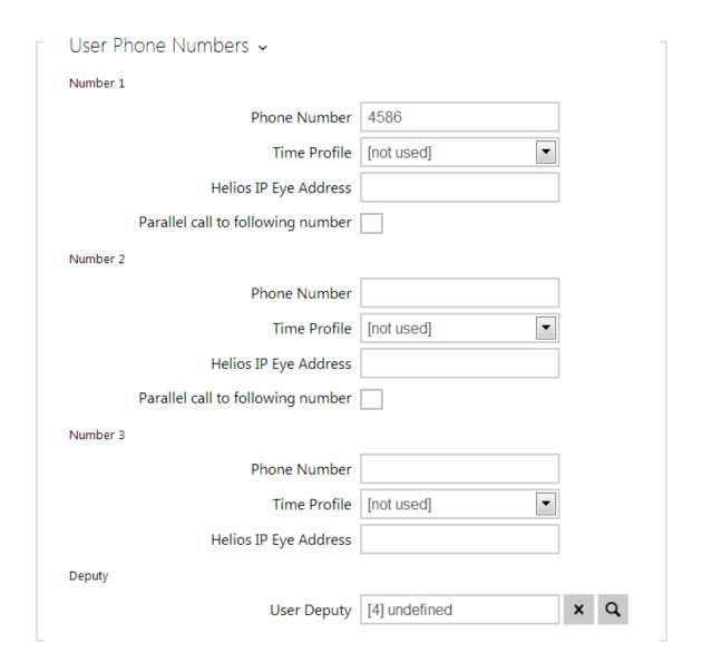
You can assign up to three user phone numbers to each Phone Book position. In case the user is inaccessible on one number, the following number will be dialled after a ringing timeout. Enable the **Parallel call to following number** to enable dialling multiple numbers simultaneously. The phone number validity can also be time profile-limited.
