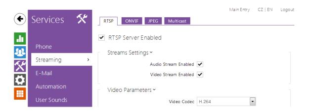
The  $2N^{\circledR}$  Helios IP intercoms provide several audio/video streaming methods; refer to the table below:
