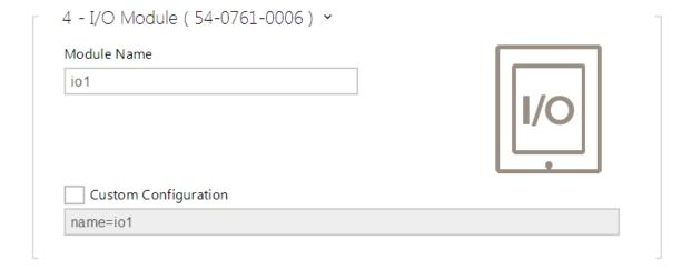
■ **Module name** – set the module name for input/output specification in the SetOutput, GetInput and InputChanged objects in **2N**<sup>®</sup> **Helios IP Automation**.
