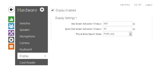
Some **2N**<sup>®</sup> **Helios IP Vario** models are equipped with a colour display. Configure the display exclusively via the **2N**<sup>®</sup> **Helios IP Manager**. In this menu, you can only switch the display on/off and set a few parameters.
