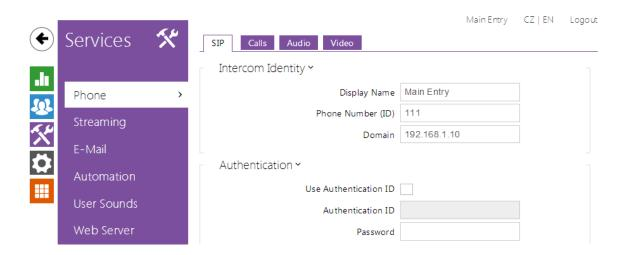
The Phone service is one of the basic functions of the intercom: helps you establish connections with other IP network terminal equipment. The **2N**<sup>®</sup> **Helios** intercoms support the extended SIP and are compatible with and certified by the leading SIP PBX and terminal equipment manufacturers (CISCO, Avaya, Broadsoft, etc.).
