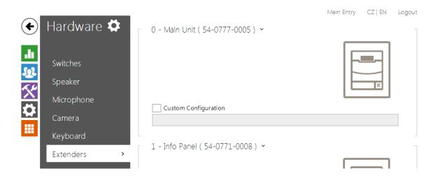
The **2N**<sup>®</sup> **Helios IP Verso** intercoms can be enhanced with extending modules connected to the intercom basic unit. The following modules are available:
