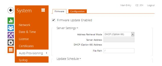
The  $2N^{\otimes}$  Helios IP intercoms help you update firmware and configuration manually, or automatically from a storage on a TFTP/HTTP server selected by you according to predefined rules.
