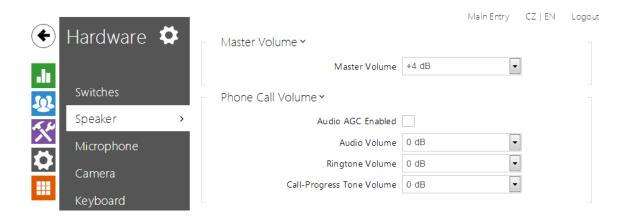
All the **2N**<sup>®</sup> **Helios IP** models are equipped with a speaker or power amplifier output to which an external loudspeaker can be connected. Set the phone call and state signalling volume control in this configuration section. The speaker volume settings are closely associated with the microphone sensitivity parameters as explained below.
