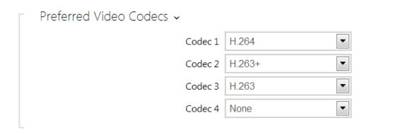
■ **Codec 1–4** – set the order of video codecs for call setup: G.711 (PCMA or PCMU), L16 or G.729. The order defines the codec priority, i.e. the first codec has the highest priority. Codec G.729 is available in selected intercoms only with a valid licence G.729.
