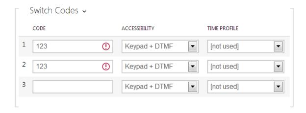
Enable the switch in the **Switch Enabled** parameter in the **Hardware Switches Switch 1** tab, set the **Controlled Output** to the intercom output to which the electric door lock is connected. Now set one or more activation codes for the electric door lock switching.
