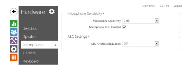
Set the microphone and line audio input volume parameters in this intercom configuration section. The microphone volume settings are closely associated with the speaker sensitivity parameters and intercom installation site conditions, which affect the general audio reproduction and recording quality. If you notice a deteriorated audio quality, please read the **Speaker** subsection carefully too to set the intercom audio parameters on your installation site properly.
