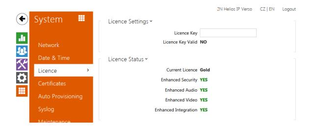
Some **2N**<sup>®</sup> **Helios IP** functions are available with a valid licence key only. Refer to the **Model Differences and Function Licensing** subsection for the list of intercom licensing options.
