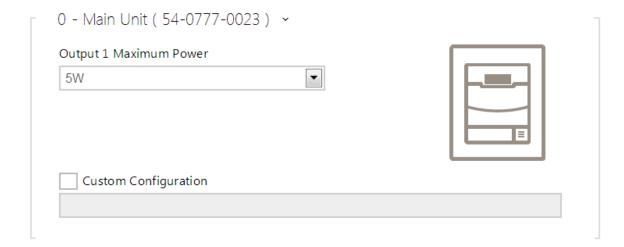
Output 1 maximum power - set the maximum load to be connected to the power output available on the basic unit. When the output is active, the consumption of the other modules (backlight level, etc.) can be adjusted automatically in order that the maximum allowed consumption of the intercom cannot be exceeded.
