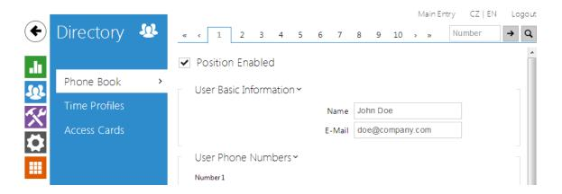
The Phone Book is one of the crucial parts of tehe intercom configuration. It contains user information relevant for such intercom functions as quick dialling, RFID card/code door unlocking, missed call e-mails and so on.
