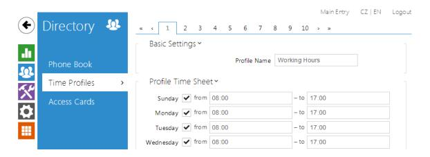
Such intercom functions as outgoing calls and RFID card/numeric code access, for example, can be time-limited by being assigned a time profile. By assigning a time profile you can:
