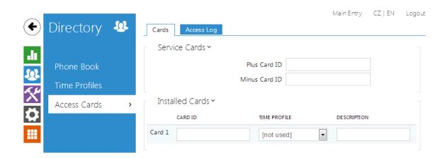
Each intercom user can be assigned one or more access RFID cards. Typically, the card ID is included in the Phone Book together with such user data as phone numbers, E-mail address and so on. Or, you can define the RFID cards in the Installed Cards list, which defines a limited number of unassigned cards reserved for visitors, for example.
