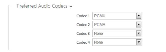
■ **Codec 1-4** – set the order of audio codecs for call setup: G.711 (PCMA or PCMU), L16 or G.729. The order defines the codec priority, i.e. the first codec has the highest priority. Codec G.729 is available in selected intercoms only with a valid licence G.729.
