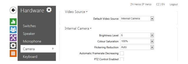
This menu is only available in the **2N**<sup>®</sup> **Helios IP** models that are equipped with an internal camera or can be connected to an external camera. The camera signal can be streamed directly into the call via a videophone, sent by E-mail, streamed via ONVIF/RTSP to another device (a video surveillance device, e.g.), or simply HTTP downloaded from the intercom in the JPEG format.
