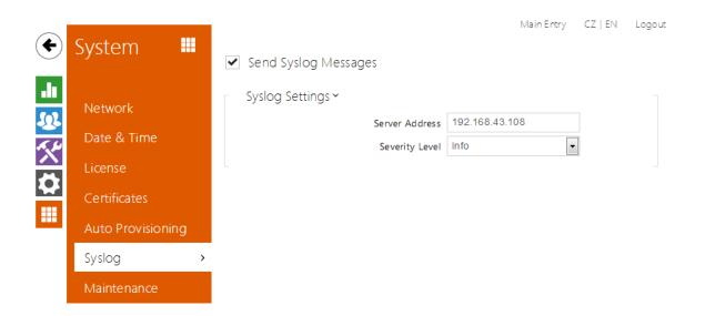
The  $2N^{\circledR}$  Helios IP intercoms allow you to send system messages to the Syslog server including relevant information on the device states and processes for recording, analysis and audit. It is unnecessary to configure this service for common intercom operation.
