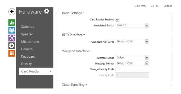
This menu is available in the 2N<sup>®</sup> Helios IP Vario and 2N<sup>®</sup> Helios IP Force models only. Configure the 2N<sup>®</sup> Helios IP Verso card reader in the Extenders menu.
